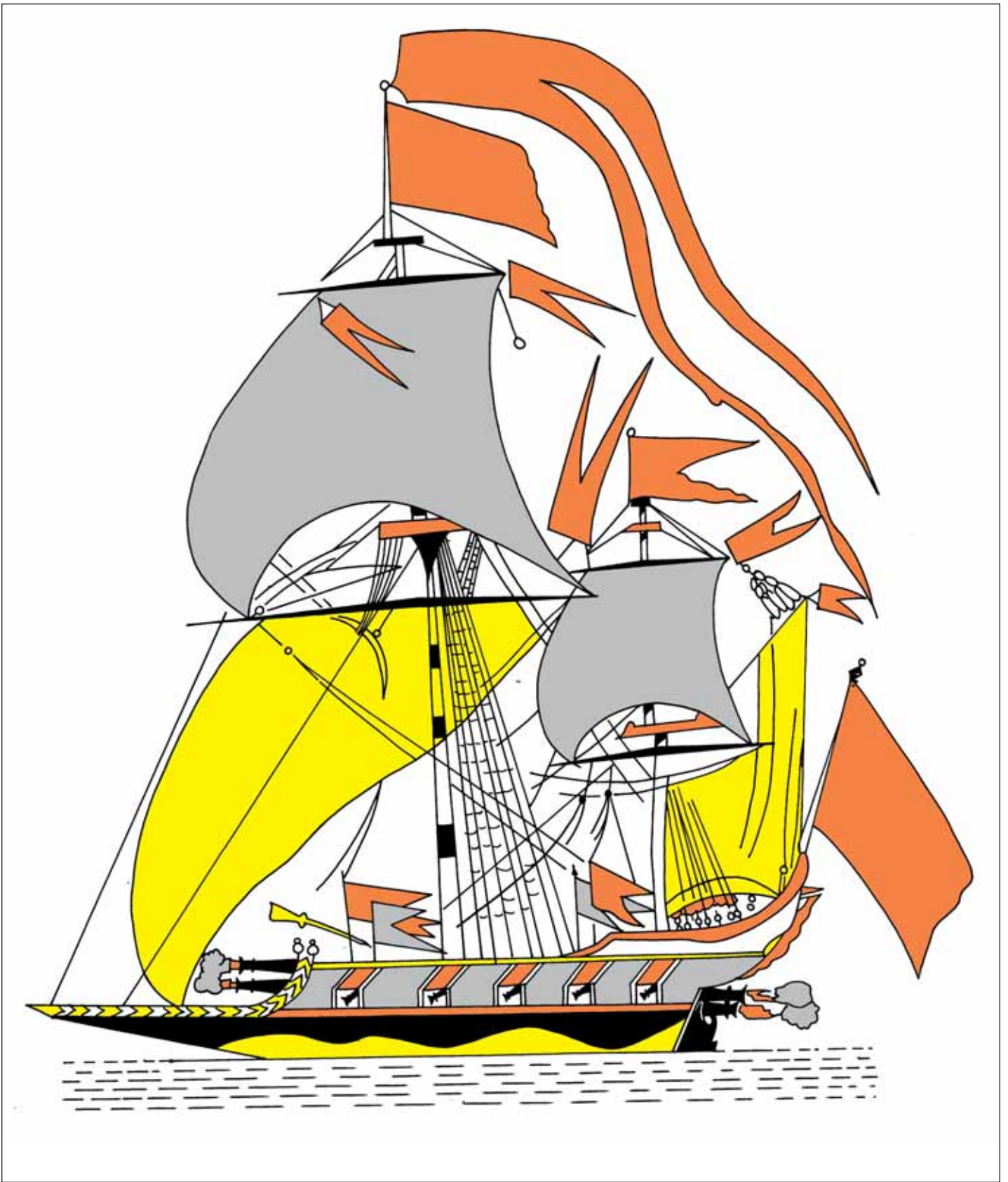
The gurab is well-equipped with cordage pulley and square sails. The masts are perpendicular to the hull and have two pieces. The fore-mast has a graceful ensign flowing from its top, so favourite with the Marathas.
