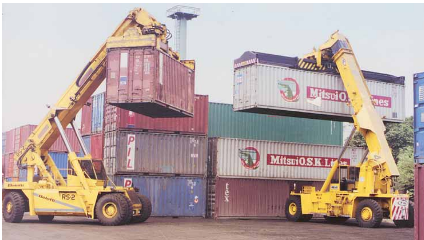
Container handling with heavy lift Reach-Stackers in Rail Container Dept., at Cotton Green
