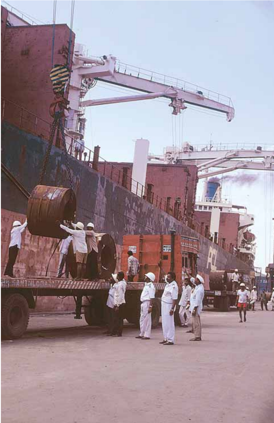
Unloading a consignment of steel rolls directly on trailers, with a heavy lift crane.
